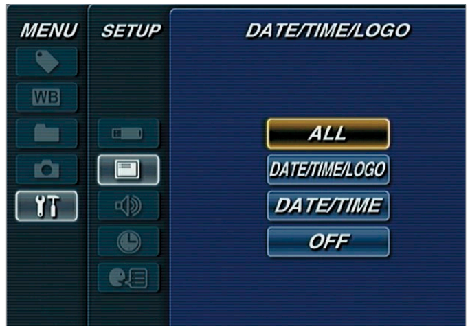
The IPLEX RX intuitive menu shows the options for image overlay
